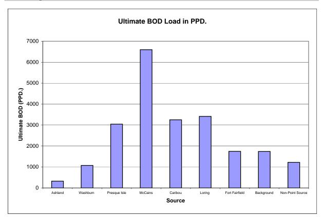
Figure 17 Ultimate BOD Loads to the Aroostook River at 7Q10 Flow
